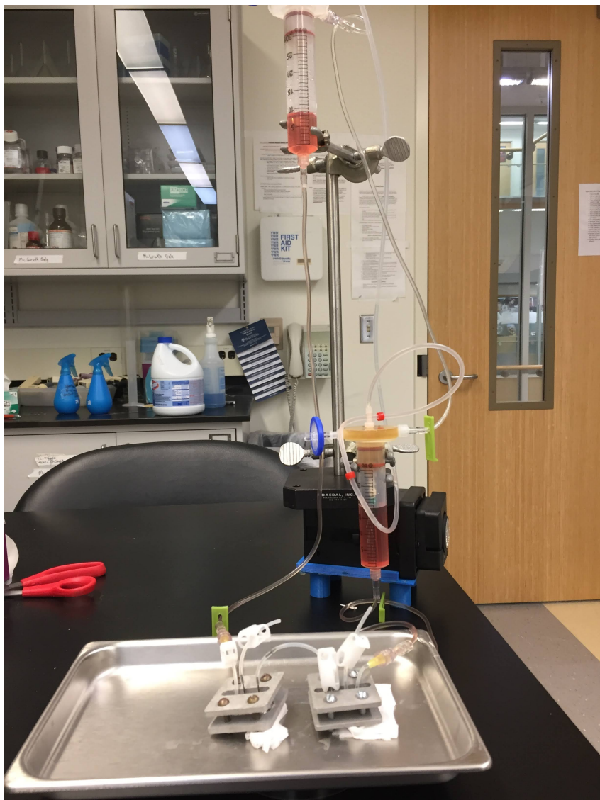
Two Alines hooked to our flow system Reservoirs ~ 14 inches apart. Placed in cell culture incubator
