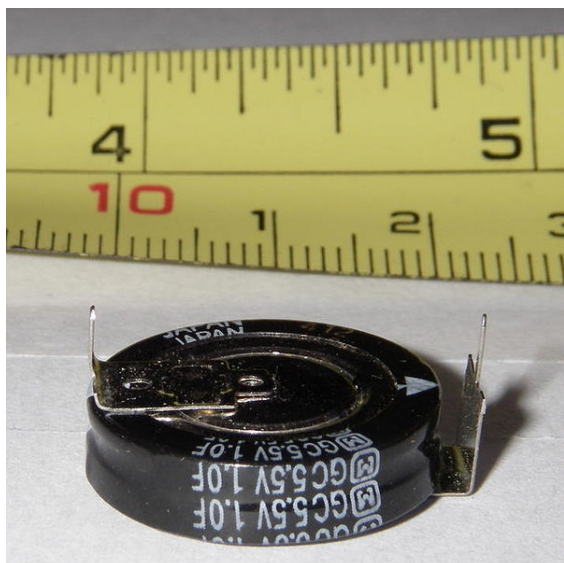
A supercapacitor with 5.5 volts is constructed out of two single cells 2.25 volt each in series connection
