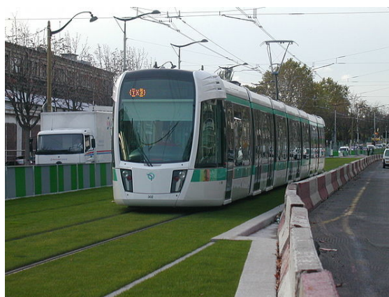
The Paris T3 line runs without catenary overhead wires in some sections
