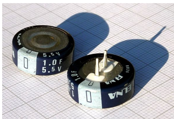
A negative bar on the insulating sleeve indicates the cathode terminal of the capacitor
