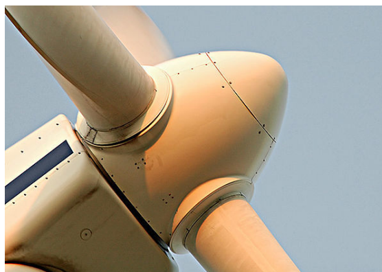
Rotor with wind turbine pitch system
