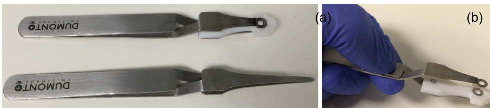
Figure S7 (a) Photograph of DUMONT crossover tweezer as supplied by Agar scientific (bottom) and modified tweezer to hold the free standing gold membrane together with the TEM grid (top). (b) The photograph illustrates the open device used to hold and press together the gold membrane and TEM grid before washing away the epoxy layer.
