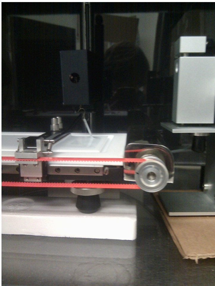
Figure S17. Image showing the existent to which the wilhelmy plate can be deflected during the course of a Langmuir experiment if a single barrier trough is used. If the surface is aspirated after compression the plate will fall back to normal position.
