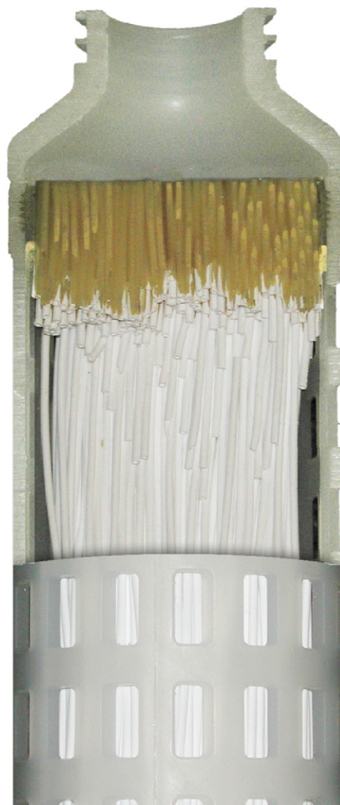
Fig. 7. Autoclavable hollow fiber cartridge with: (1) annealed polypropylene to eliminate polymer stress; (2) smaller diameter to reduce thermal expansion and contraction; (3) serrated bonding surface between polyurethane potting compound and polypropylene cartridge; (4) increased thickness of cartridge cage; and (5) inserted metal ring in cartridge outlet (not shown) to stabilize seal during heating and cooling. Photo used with permission of Genentech, Inc.
