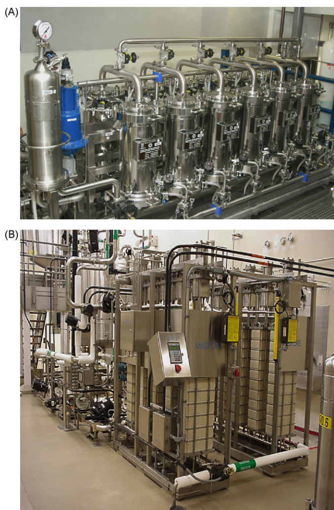
Fig. 9. Large-scale microfiltration systems for harvest of recombinant DNA derived proteins from Chinese Hamster Ovary Cells. (A) Microdyn 0.2 \mu\text{m} polypropylene hollow fiber microfiltration system with 174 \text{m}^2 membrane area. (B) Millipore Prostack™ flat sheet membrane system with 186 \text{m}^2 of 0.65 \mu\text{m} pore size hydrophilic PVDF membrane. Photos used with permission of Genentech, Inc.
