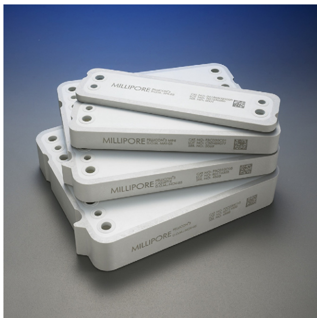
Fig. 17. Linear scale ultrafiltration cassettes with constant channel length and mass transfer coefficient (same turbulence promoting screen and channel compression) can provide thousand-fold linear scale-up of ultrafiltration processes. Twenty-thousand-fold linear scale-up is possible with new linear scale devices such as Millipore Pellicon® 3 cassette. Photo used with permission of Millipore Corporation.
