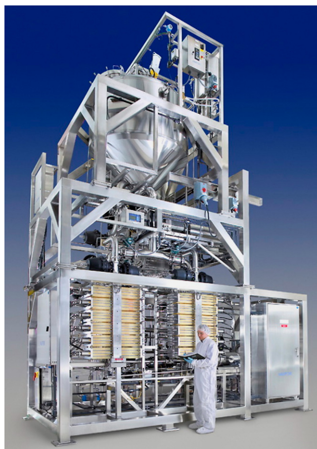
Fig. 18. High concentration UF system with 250 m 2 membrane area. New tank design with a retentate lift tube combined with close-coupling of all feed and retentate components in a vertical arrangement resulted in a minimum operating volume (including product in the recycle tank) while maintaining good mixing, minimal short-circuiting of retentate to feed, and no air entrainment. Photo used with permission of Genentech, Inc. and Millipore Corporation.
