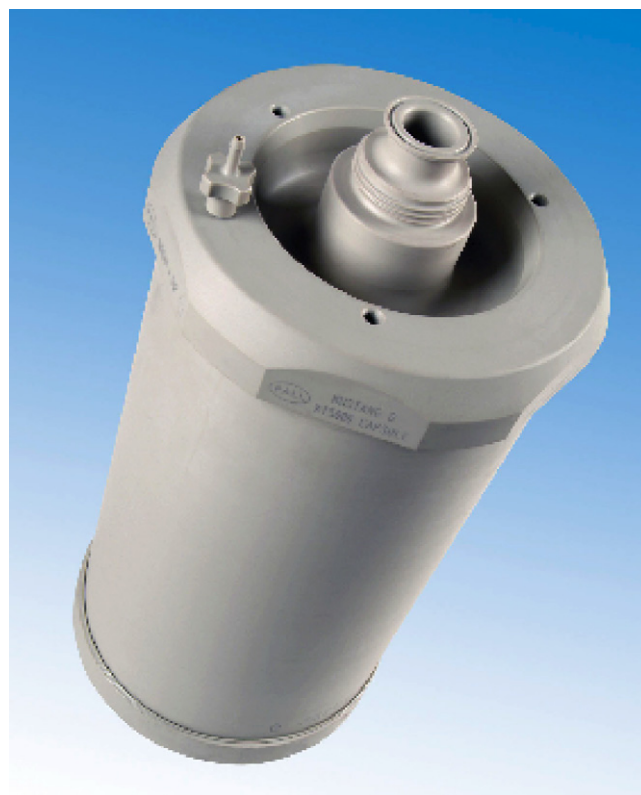
Fig. 12. Industrial scale membrane chromatography unit. Pall Mustang® 5 L XT 5000 module with 16 layers of pleated 0.8 \mu m PES membrane with quaternary amine ligand. Photo used with permission of Pall Corporation.
