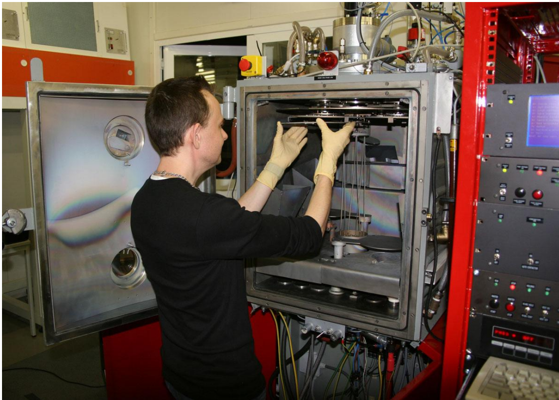
Figure 24. A retrofitted Balzers BAK 550 box coater with completely new interior and computer controller. All coatings used in this thesis were produced by this machine.
