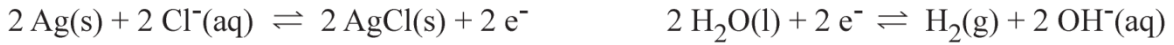
Figure 1 Diagram illustrating a hydrogen evolution in an electrolytic cell composed of a pair of Ag/AgCl electrodes in KCl solution at 25 °C, 1 bar of pressure, and pH neutral
